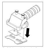
Carefully loosen the base plate from the positioning cams and remove.
