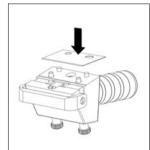
Place a new, sterile blade in the positioning cams.
