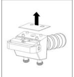
Remove the blade and dispose of it
