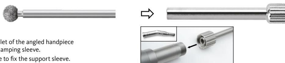
1. Insert the milling cutter shank into the open collet of the angled handpiece up to the stop. Close the collet by turning the clamping sleeve.
