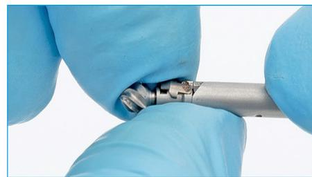
Fix burr head in place by closing the lock with your finger. Check seating with a slight countermovement.
